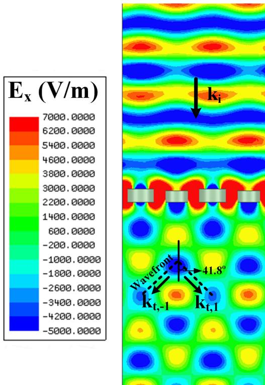
Fig. 4. Electric field distribution showing the interference pattern of the two splitted beams at the transmission side.
