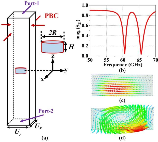
Fig. 1. (a) Typical simulation environment with periodic boundary conditions (PBC) and Floquet ports (Port-1 and Port-2). (b) Simulated magnitude of the transmission coefficient for  $R = 1.4$  mm and  $H = 1.25$  mm. (c) Electric field distribution at 60.6 GHz. (d) Electric field distribution at 65.6 GHz.
